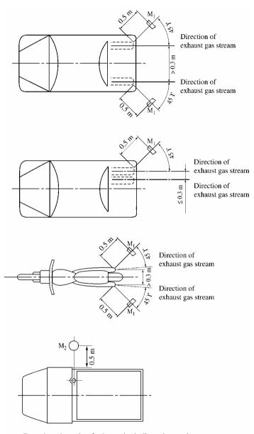
Case where the outlet of exhaust pipe is directed upwards
